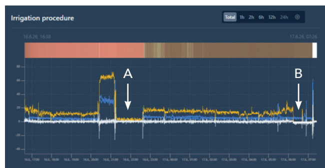
Figure 1: Irrigation course documented by filaxONE. A) Temporary irrigation interruption. B) Discrepancy between inflow (blue) and outflow (orange).
