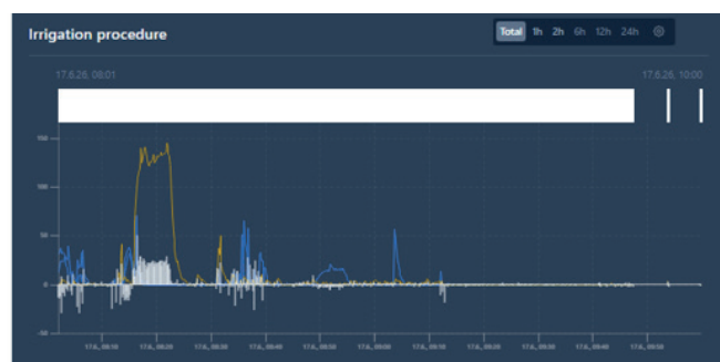
Figure 2: Irrigation course documented by filaxONE after removal of the obstruction. Inflow (blue), outflow (orange).
